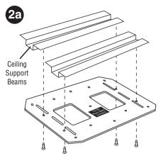
Mount support bracket using screws (not supplied) with the "This Side Mounts Against Roof/Ceiling" label against ceiling support beam(s).
